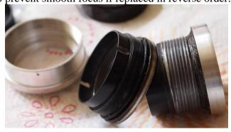
With the guide pins out, the inner helical unscrews. The grease is usually dry, and needs to be removed completely. Save those old tooth brushes and dip them in alcohol or lighter fluid. The inner helical can be dropped in an ultrasonic cleaner if you have one.
