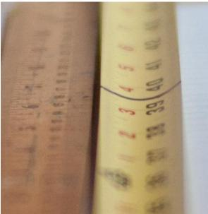
This is about as good as I can get an F1.5 lens on my Leica M8 and M9. You will need to reshoot the ruler, adjust the thickness of the shim accordingly. Reduce the shim slightly if it is now front-focusing, and thicken it a little if it is still back-focusing. The amount of residual error is an indicator of focus deviation from 52.4mm.
