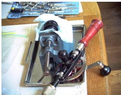
The tape is to keep the aperture ring from moving as you tap out the holes. Do them sequentially; some trial and error might be required. Once the holes are done, put the set screws back into place. If they are not flush, remove and drill deeper. At this point, put
