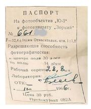
The focal length is given as 52.4 +/- 1%. That gives a range of about 51.9mm to 52.9mm. Those on the short end of the range will work well on a Leica. The average will work well once the main shim is adjusted, and those on the upper end will require the focal length to be reduced and then the main shim to be adjusted.
