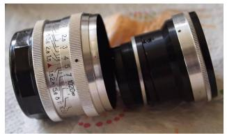
The shim is the aluminum ring that controls the stand-off between the optics and the RF Cam of the inner helical. This, and exact focal length of the lens, controls agreement with the camera's RF. To achieve critical focus at F1.5 an accuracy of 0.02mm is required for
