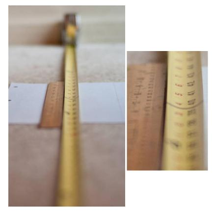
For this case, the RF of the camera was focused precisely on the 1m mark. I lined the metric ruler up with "16cm" straight across from the 1m (39.4") mark on the tape measure. The actual focus is between "19cm" and "20cm", meaning the lens is backfocusing by about 35mm.
