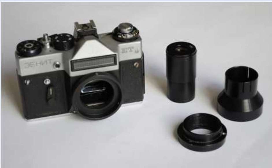
"A" coupler in camera, Ocular 14x, M42x1 Cannon, "A" ring, Barlow Lens Retainer.
